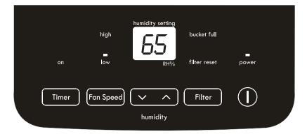
5. The FILTER RESET light will illuminate after 250 hours of operation. At this time, refer to the "Care and Cleaning section to remove and clean the filter. Once the filter has been cleaned, simply press the FILTER button to extinguish the light.
